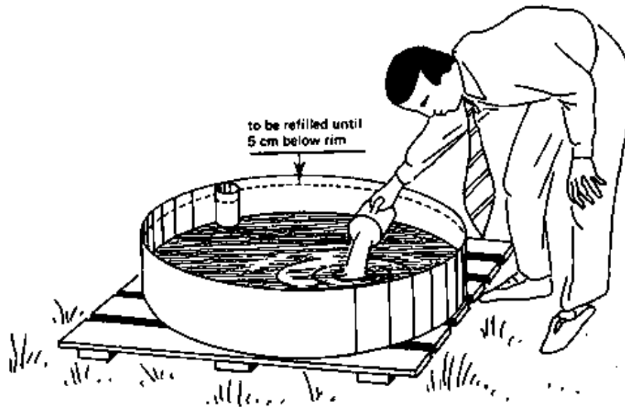
Fig. 9b Take water out of the pan when the water depth rises too much
